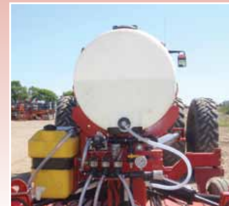
Liquid Applicator System for weed control while mowing
