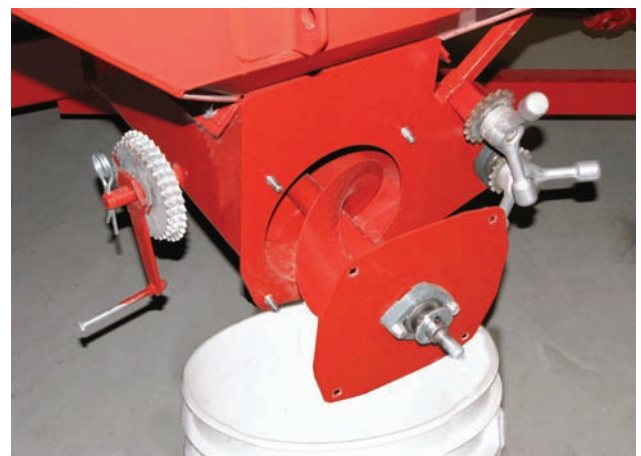
Pull Out Auger To Drain Tank
